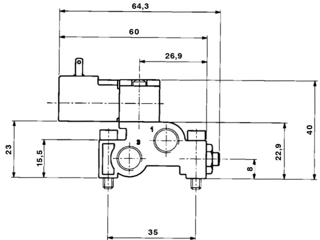
1 = Speisung      3 = Entlüftung **Ventile NC**
