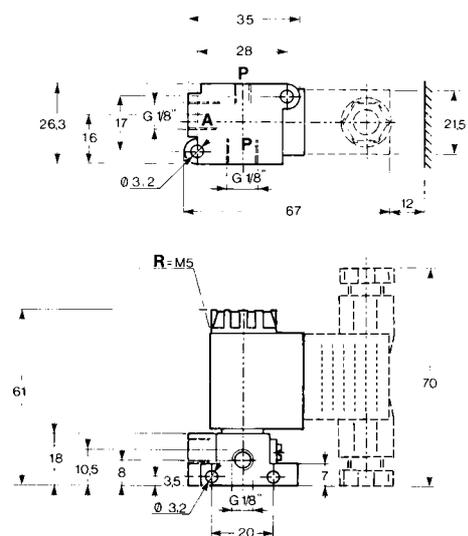
**PILOTVENTIL U1, Gewindeanschlüsse M5**
